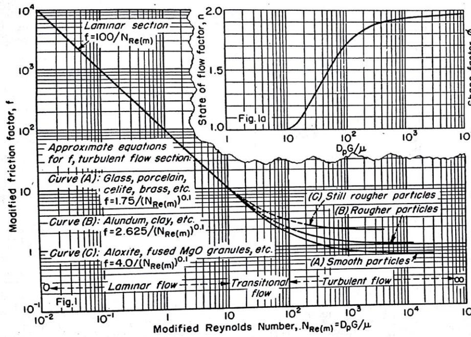
Fig. 1—Modified Reynolds number-friction factor plot for packed beds.
